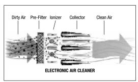
This illustration shows how a duct-mounted electronic air cleaner, directly connected to a home's heating and air cooling system, cleans the recirculated air.
